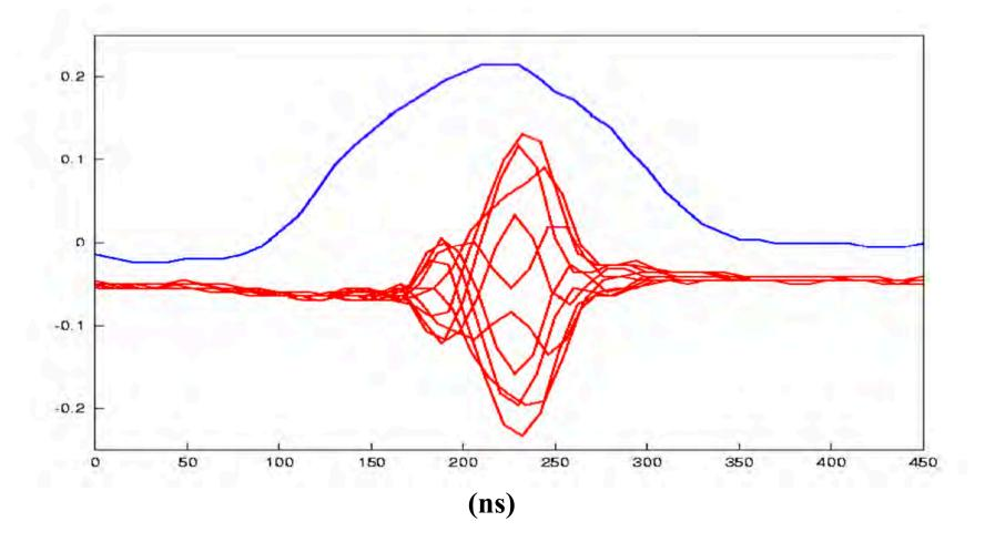
BPM signals: sum (blue) and difference (red). The instability caused emittance growth and was self limited after some beam loss. 24 Haixin Huang BROOKHAVEN
