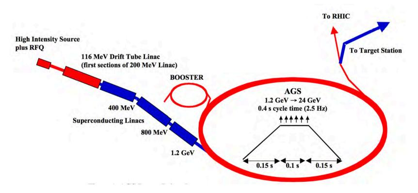
Increase AGS average beam power from 0.2MW to 1MW. It requires power supply and RF upgrade for faster ramping in additional to the 1.2GeV superconducting linac. This was proposed in early 2000, but never proceeded.
