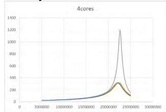
J-PARC cores (10µm thick) also gives a high impedance at 20 MHz !
