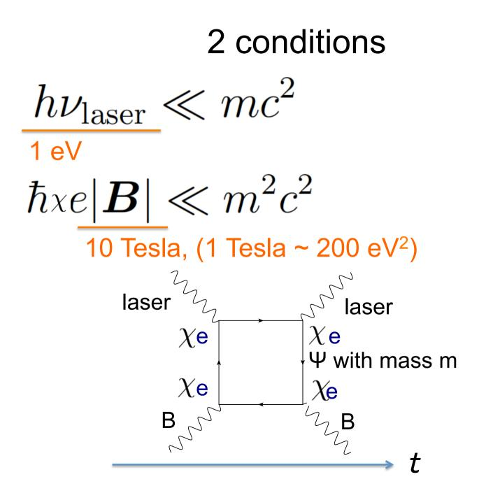
Vacuum Magnetic Birefringence Experiment: laser beam energy
