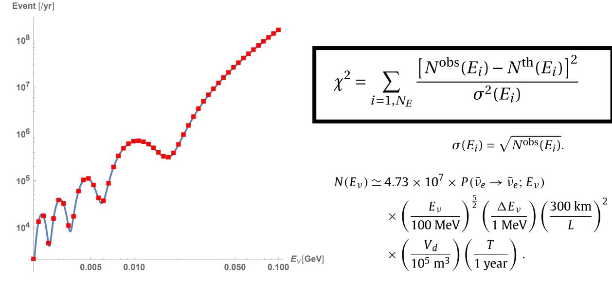
4. We determine those density by minimizing the  $\chi^2$  function by comparing the observational data  $N^{\mathrm{obs}}(E_i)$  for a given original profile  $\rho(\mathbf{x})$  with the theoretical prediction  $N^{\mathrm{th}}(E_i)$  from unknown parameters  $\rho_j$ .
