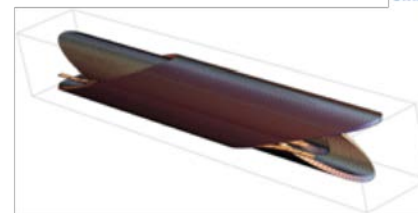
Canted Cosine Theta option for the 16-T FCC-hh main dipole (PSI)
