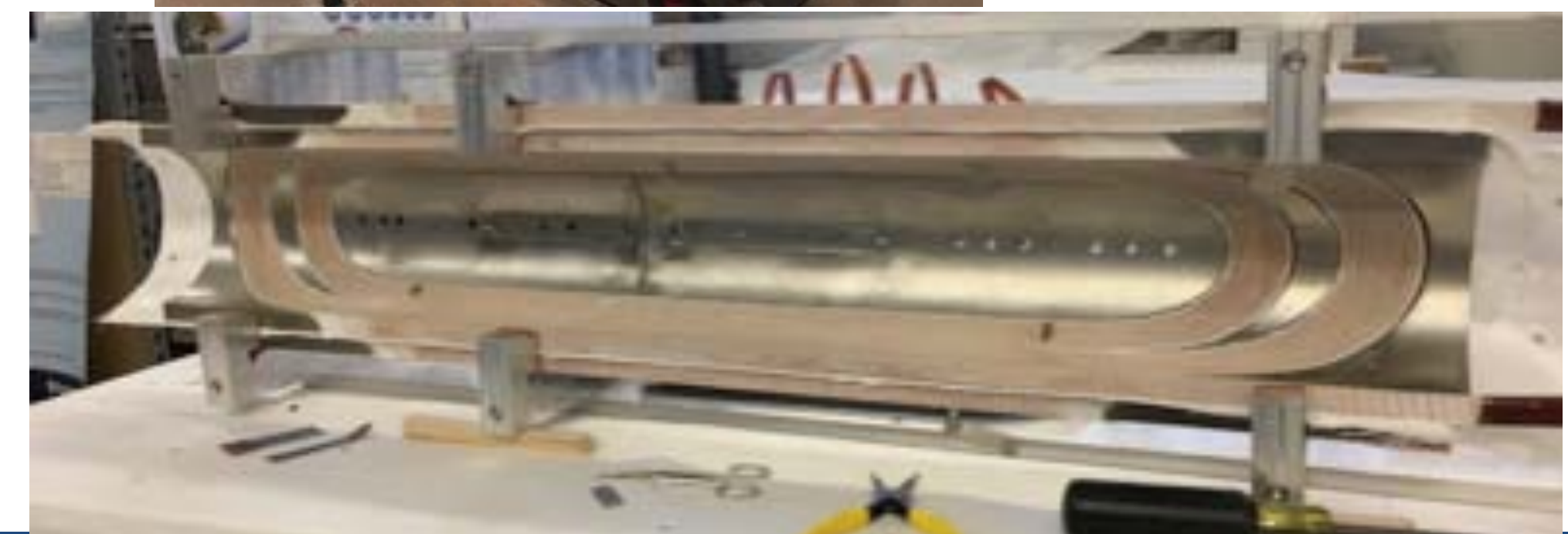
60-mm aperture, 4-layer graded coil
