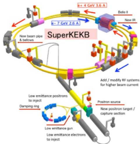
Figure 3.1 – Schematic of the SuperKEKB Accelerator [13].
