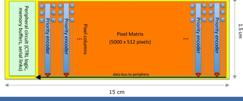
Migration of the design to Tower 65 nm  $\rightarrow$  <20 µm pixel pitch
