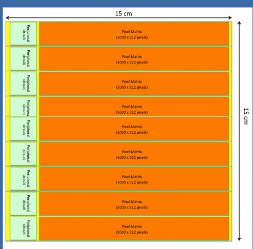
Sensor periphery contains the control logic, the interfaces for the configuration of the chip and the serial data transmitters
