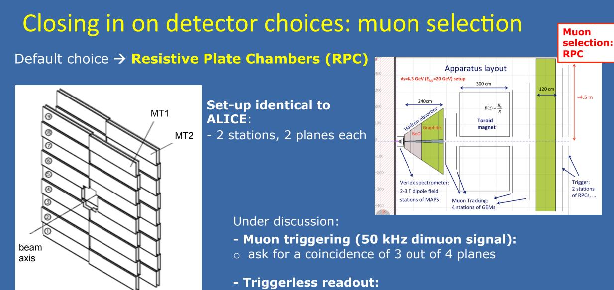
• All collisions are readout; RPCs used for muon identification
