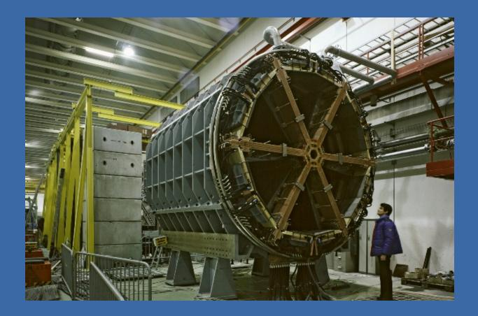
**NA60 used the ACM**, an open toroid with field circling the beam-axis with an excellent field quality
