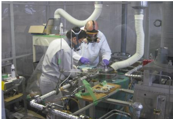
SNS gas wall experiment using mercury cavitation device in J-PARC (2009)
