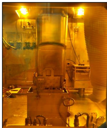
Robotic device to cut target vessel samples
