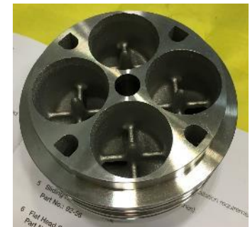
SNS swirl gas bubblers, leverage Japanese development (2018). This will enable SNS to operate at 2 MW after PPU.
