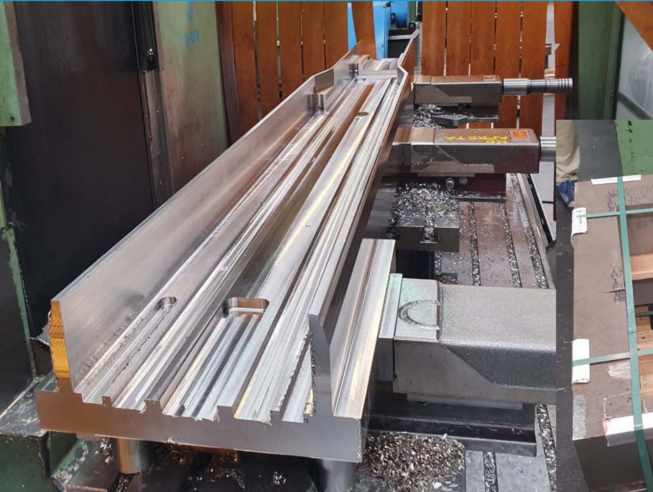
Bottom part of port tube, with insert alignment features
