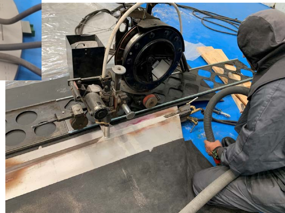
Vessel bottom plate fabrication through submerged arc welding technique
