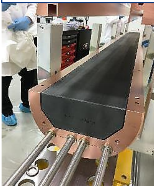
TIDVG 4 core being pulled into the vacuum chamber
