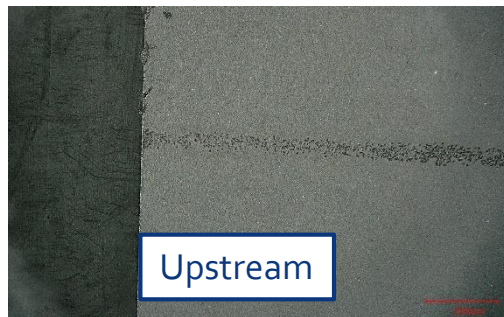
Surface damage detail in Mo coating: tilted impact
