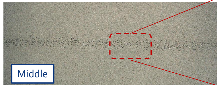
Surface damage detail in Mo coating: tilted impact
