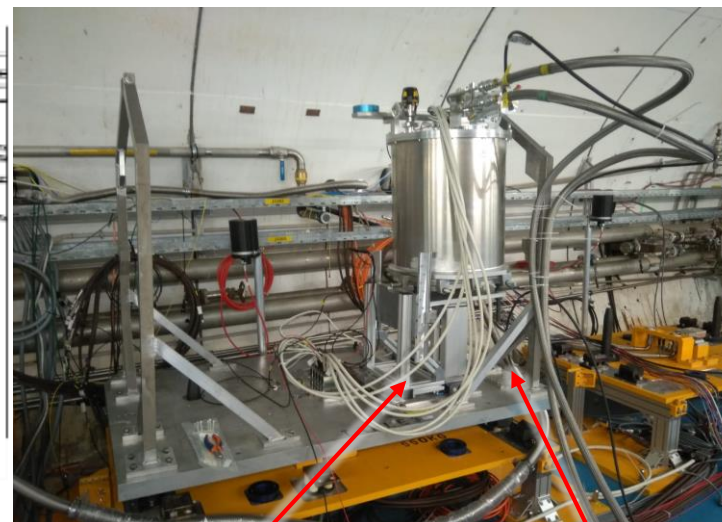
horizontal stage \Delta x = 330\text{mm} Accuracy \pm 300\mu\text{m}
